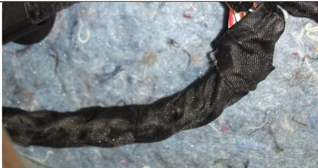
I cut all four black wires and the white / violet one. Don't do this too close to the bracket, or too close to the sheath opening. You will want room on both sides to work with.
