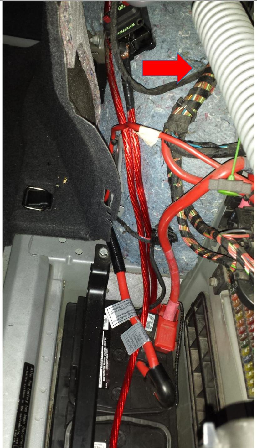
At the top of the wheel well, I ran it into some foam and then across the top trunk conduit. (this is the view from seat folded down)
