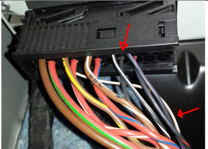
All of these wires have a sheath on them. You will need to carefully cut back the sheath, at least around the bottom loop.
